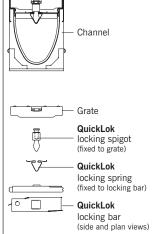
ACO **QuickLok** is a patented boltless locking system, grates are removed and replaced with the minimum time and effort for ease of maintenance. The unique design provides a positive 'snap down' fit into the locking bar. A spigot is fixed to the grate which 'locks' into the spring in the locking bar.
